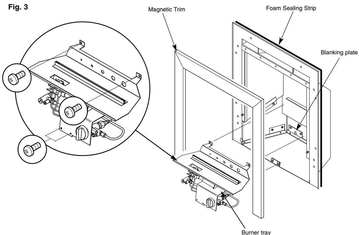
9. When the burner tray has been removed, decide which side of the appliance the gas supply will be entering the radiant box and remove the relevant blanking plate. The gas supply should be concealed as much as possible. Both blanking plates **MUST** be re-fitted or this could seriously impair performance.
